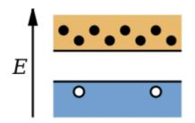
Band structure of an n-type semiconductor. Dark circles in the conduction band are electrons and light circles in the valence band are holes. The image shows that the electrons are the majority charge carrier.
