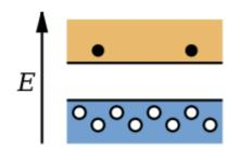
Band structure of a p-type semiconductor. Dark circles in the conduction band are electrons and light circles in the valence band are holes. The image shows that the holes are the majority charge carrier
